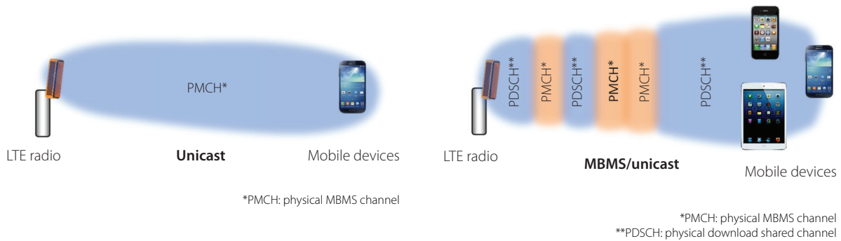
Figure 3. Unicast (PDSCH) and broadcast (PMCH) transmissions
