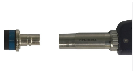
The Sidewinder will automatically inspect all 12 of the fibers in the Q-ODC-12 connector
