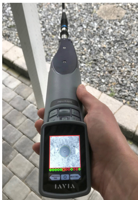
Sidewinder™ inspecting a Q-ODC-12 Plug
