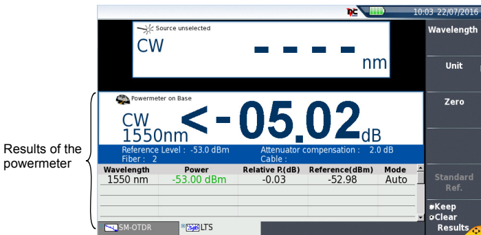
Fig. 19 Results and commands of the power meter
